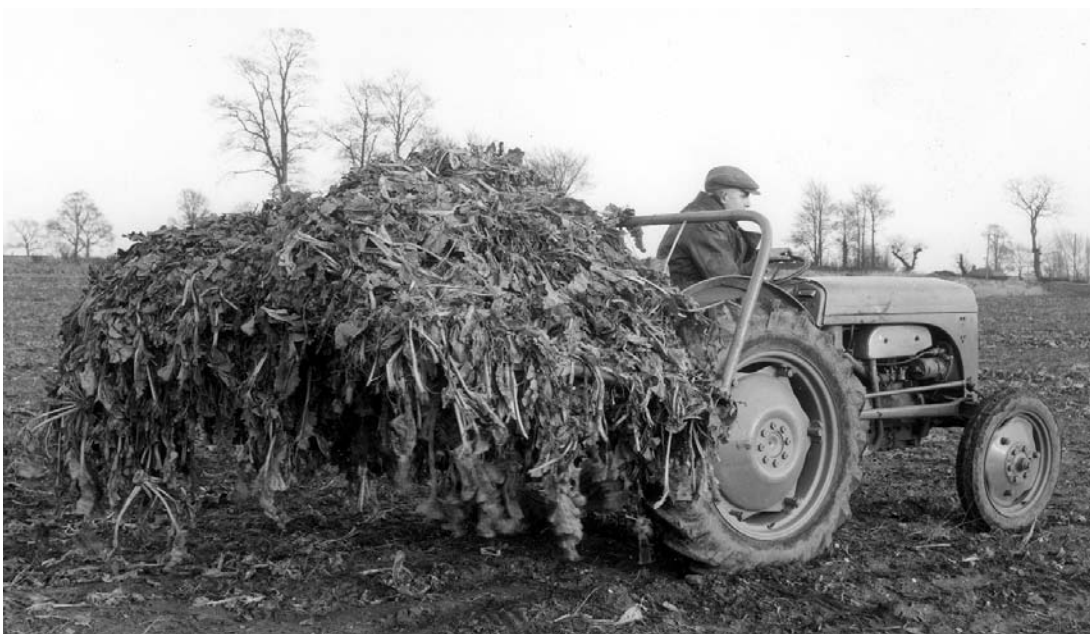
The Ferguson buck rake being used on a cold winter's day. Note the drive for the Tractormeter adjacent to the dynamo.
