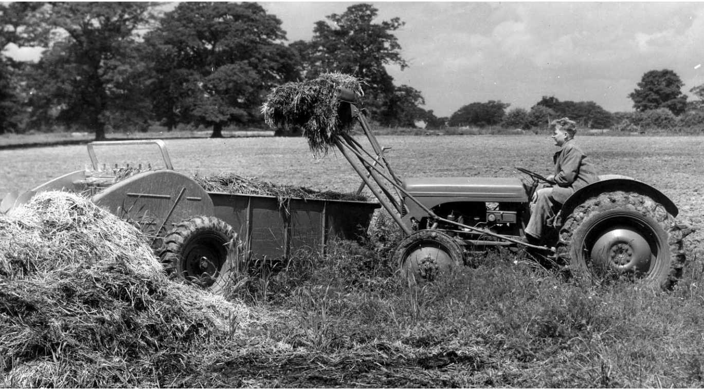
A TE.H20 with the early-type loader L-VE-20 being used to fill a manure spreader type A-IE-A20.
