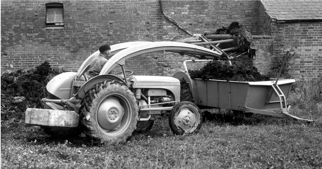
A TE.D20 fitted with the high lift loader M-UE-20, commonly known as the banana loader, doing the same job. Note the rear concrete weight.
