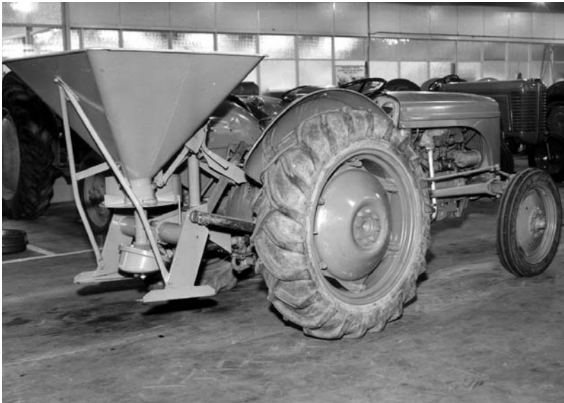
A photograph taken in the Fletchamstead Highway engineering shop of the Massey-Harris-Ferguson mounted spinner broadcaster FE30 (721). What looks very much like an LTX is lurking in the background.
