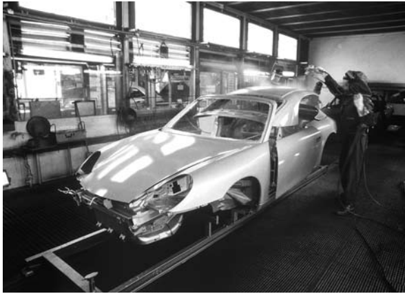
A 996 Cabriolet being hand-painted just like all the previous series. Notice the hardtop being painted at the same time, which ensures a perfect match. Contributor: Dr. Ing. h. c. F. Porsche AG
