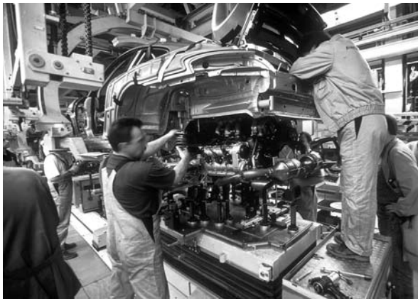
The 996 production line with lots of hands on deck, and not a robot to be seen anywhere. Looks hand-assembled, just like the 964 and 993. Contributor: Dr. Ing. h. c. F. Porsche AG
