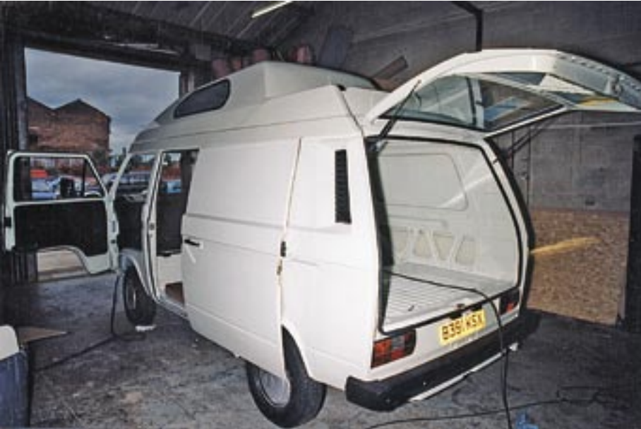
2-2-1. This T3 Transporter van has already had its new high-top roof fitted and is now ready for the side windows to be fitted.
