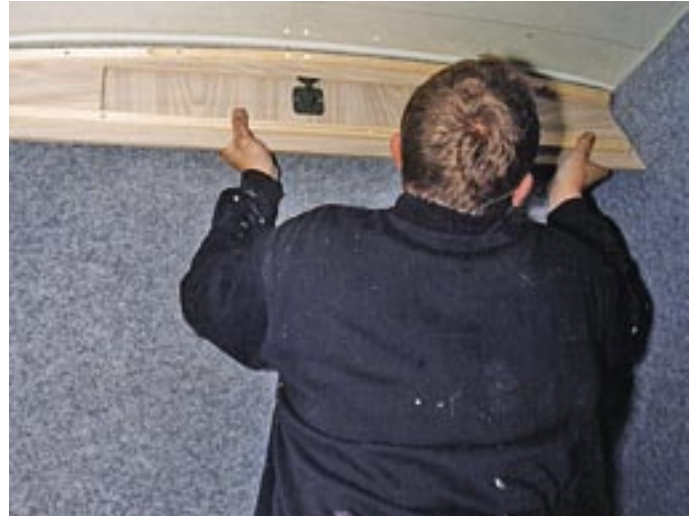
2-4-15. Back on the Volkswagen T3, Barry is fitting the shallow cupboard at the rear of the van's steel roof.
