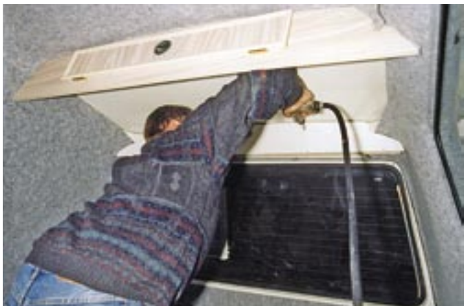
2-4-16. There are no brackets in this case, so Barry drills through the strut on the cupboard and into the rib which runs across the roof.
