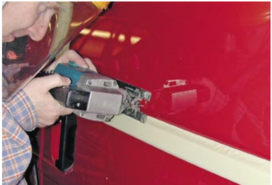
2-2-18. Wearing the obligatory eye protection, Barry cuts carefully to the outer of the two pencil lines.
