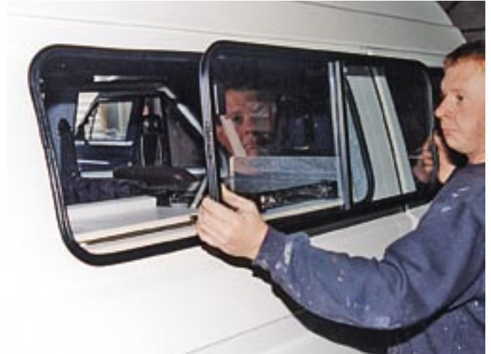
2-2-28. Barry P fits this sliding glass panel, which is done in a completely different way, the surround being fitted to the bodywork first.
