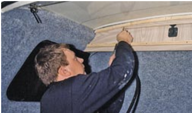
2-4-16. There are no brackets in this case, so Barry drills through the strut on the cupboard and into the rib which runs across the roof.
