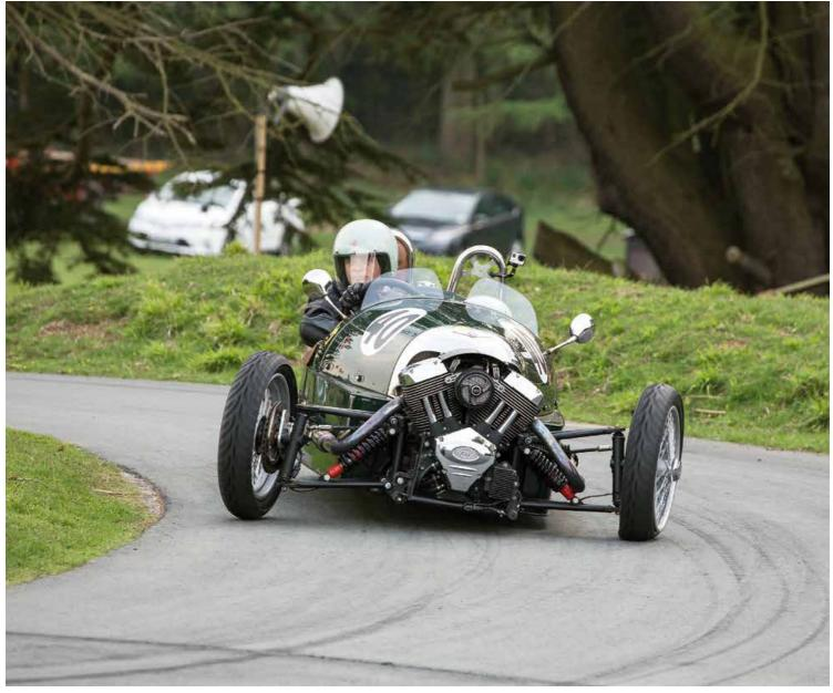
Reeves' highly modified 2012 M3W, with 128in<sup>3</sup> engine, reduced ride height, adjustable dampers, smaller wheels, and no mudguards. Note the slip angle of the loaded tyre. (Courtesy Jay Stride/MMC)
