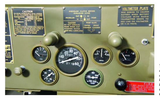
The dials are standard GPW but the instructions above the speedo tell the driver how to use the two levers for propeller and bilge pump – not something a driver on a GPW normally had to worry about. Below the volt meter the large black shiny knob is for the winch control on the front. Pushed in like this it kept the winch disengaged while pulling it fully out engaged the winch.
