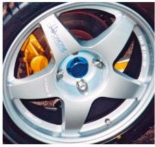
10-6 The brake caliper clearance offered by these superb Compomotive wheels is exemplary. The rims are 7in and are running 205 x 50 x 16in tyres, while also showing off the brake calipers (in this case SD1 Vitesse).
