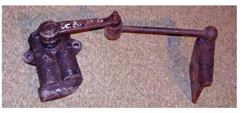
7-1-1-1 The original Armstrong lever arm damper, its connecting link, and spring pad – all of which are discarded when replaced by the much more effective telescopic dampers.
