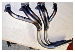
3-4 The MGC exhaust manifold/header. It is preferable but not mandatory to fit a twin-pipe/twin-box exhaust system at the first opportunity ... although, to be fair, you will not loose much power and will be hard pushed to detect the difference if you retain your standard single-pipe/box system, at least until it comes time to replace the exhaust system.
