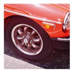
10-5 These are the more usual bolt-on Minilite wheels but this time finished in 'Slate.' The polished rims require some additional maintenance in that without care their surface will corrode.
