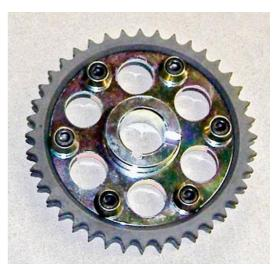
3-5 An MGC vernier timing sprocket bolts to the camshaft, of course, which reminds me to mention that new camshaft blanks are not now being produced. As a result, you'll need a good, straight camshaft to trade-in if/when you seek an uprated one.
