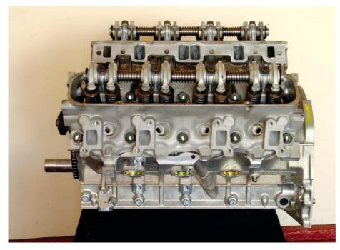
4-2-3 The 4600cc cylinder blocks have five pairs of cross bolts that go through the blocks into the sides of the main bearing caps.
