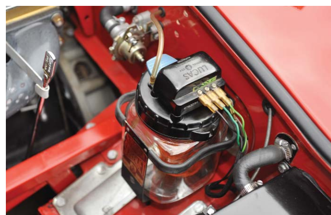
The windscreen washer has a square-section glass bottle. To the left is the dipstick, with the handle marked “Stop engine – wait 1 minute”, and between the two is the water valve for the heater.
