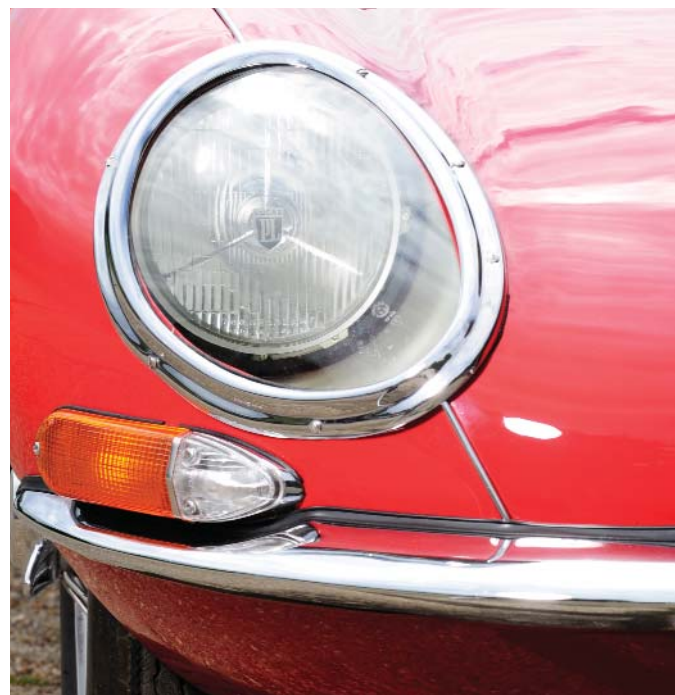
The Lucas PL700 headlamps have a tripod with central reflector bearing the PL badge. As this is a June 1961 car, maybe it should have body-coloured headlamp buckets, while later cars typically have silver buckets. The glass covers reflect light from outside as well as inside, and water does get past the rubber seal of the chrome surround. Below is the combined flasher (amber lens) and side light (white lens).
