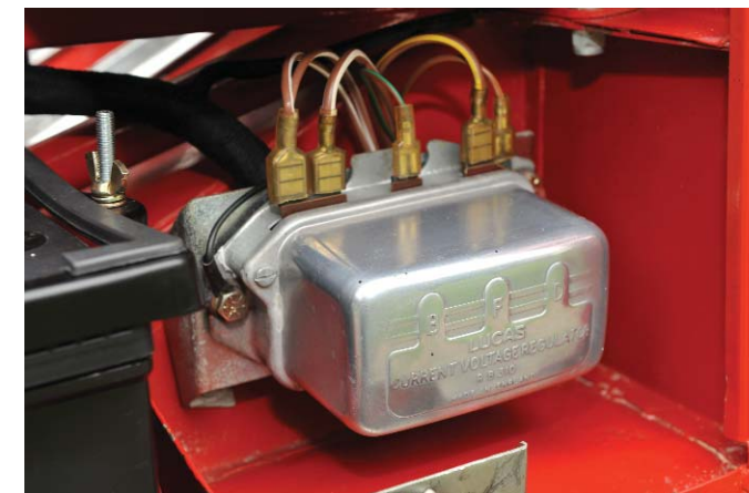
The battery and control box were mounted in the left-hand front sill, below the heater box. Early cars until August 1961 had the RB310 control box with an aluminium cover; later cars the RB340 box with a black plastic cover. Neither of the batteries shown is of the original type. Note also the two different types of bonnet lock catches, for the external and internal locks respectively.
