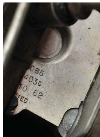
Some Lucas electrical components were date-stamped such as this wiper motor “10 62”, but also the dynamo and starter motor.
