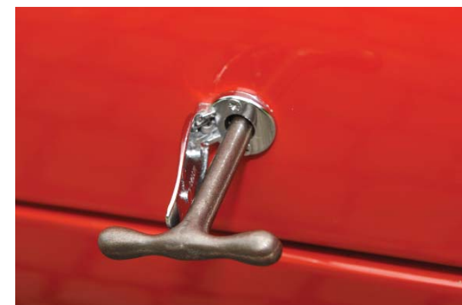
The external bonnet locks on the early cars had teardrop-shaped covers, pointing towards the rear, and were operated by a coach key. The third picture is the lock on the inside of the bonnet.
