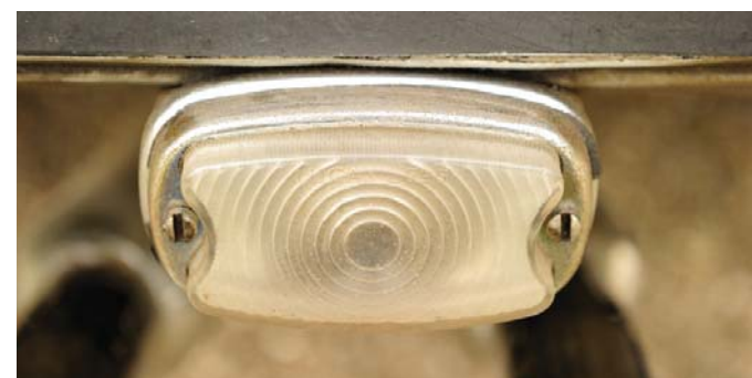
The reversing lamp sits in a chrome-plated housing in the centre below the rear number plate.
