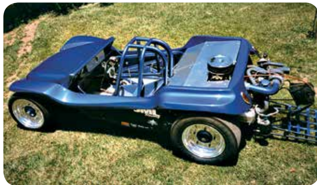
John Leso's Manx drag racer is built on a custom tube chassis, uses nitrous oxide for extra power, and Porsche brakes to stop it at the end of the quarter-mile. (Courtesy Mel Baker)
