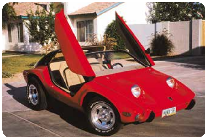
Bruce Meyers' sophisticated street buggy The Manx SR featured flip-up doors, and removable roof panel. (Courtesy Mel Baker)
