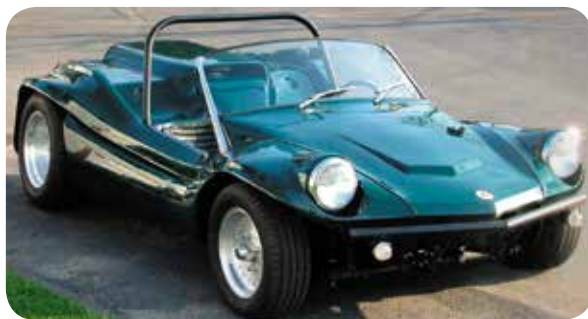
With the addition of an Autodynamics tubular chassis, the Deserter became a serious racing vehicle with mid-mounted Corvair or Porsche 911/912 engine, and was re-named the Deserter GS. (Courtesy Alex Dearborn)
