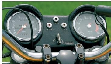
The Smiths tachometer now had a 7000rpm red line. The needle on this example is broken – a common problem with Smiths instruments.
