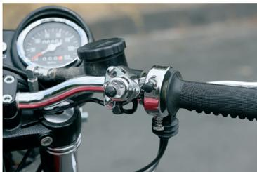
The right Aprilia indicator switch mounted on a specific triangular plate.
