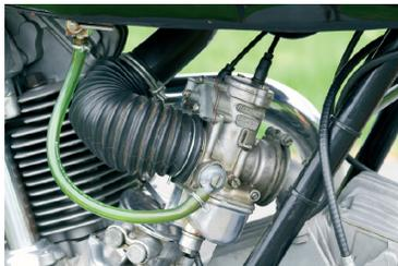
Dell-Orto PHF 30A carburetors were fitted towards the end of 1973, but the pleated plastic air intakes remained.
