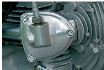
A new tachometer drive was fitted to the front cylinder head during 1973. This was for Veglia or Smiths instruments.
