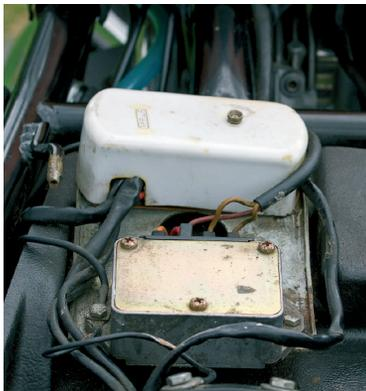
With the Dellorto carburetors the regulator moved to a plate under the seat next to the fuse box.
