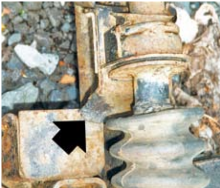
6-35-1. The TR4A steering rack (note the 'D' washers welded to the rack and the rubber cushion mounting), used, in fact, on TR4As, 5s, 250s and TR6s, with its traditional, but most undesirably cracked, mounting (arrowed).
