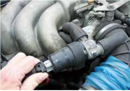
The idle valve can gum up, making the engine prone to stalling. Removing and cleaning with WD40 can revive it.
