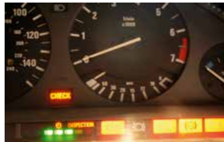
Check all the right warning lights come on as soon as the ignition is turned on, then go out when the engine starts.
