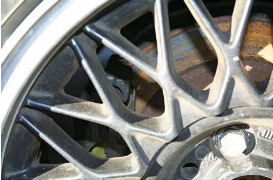
This disc has light surface rust, typical of a car that has stood for a few weeks.
