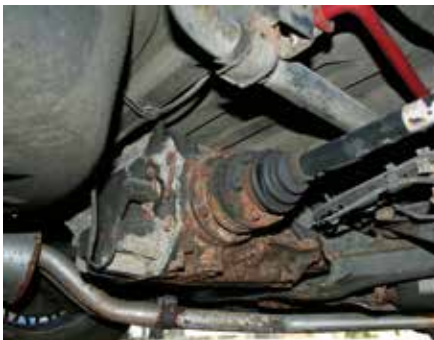
There should be no oil dripping from the front or rear. Slight oil staining from the top is due to oil mist coming out of the breather, and is usually not an issue.
