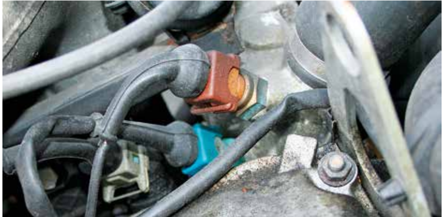
The biggest cause of problems with old fuel-injection systems are the connectors. Vibration loosens the contact's grip, and tarnishing increases resistance.
