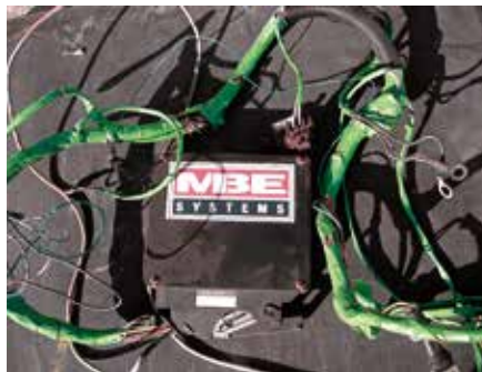
For heavily modified engines, it may work out easier and cheaper to change to a mappable ECU, such as this MBE941.
