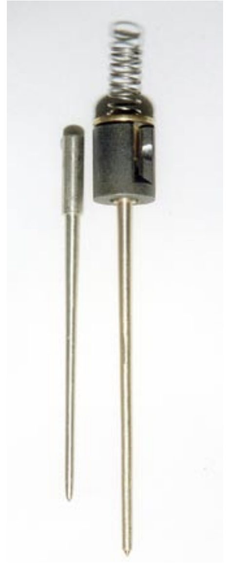
Fixed type needle on the left fits into the piston just as it comes. Spring-loaded needle needs a spring and collar, as shown on the right, before it can be fitted into the piston.
