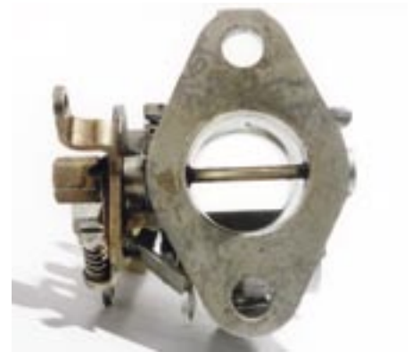
Thinned down spindle after screws have been ground down and the spindle 'flash soldered' (see text).
