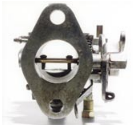
Modified SU carburettor spindle with the standard butterfly screws fitted and ready to be ground down.
