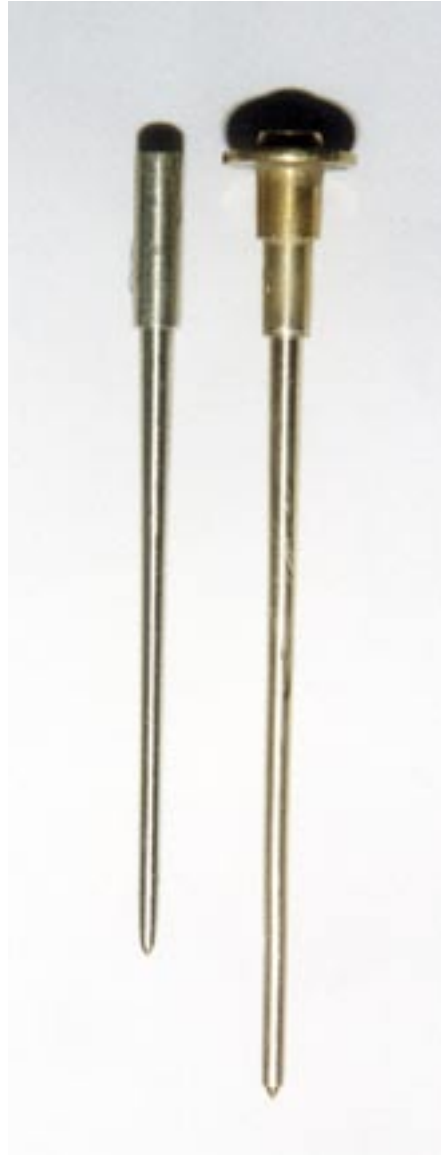
Fixed type of needle on the left and spring-loaded type on the right.
