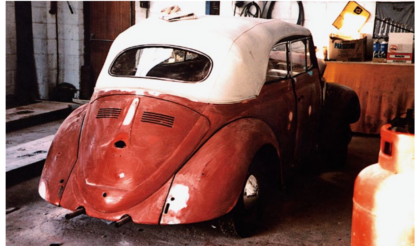
The Cabrio's air intake louvres were quite different to those of the Beetle saloon. (Courtesy Martin McGarry)
