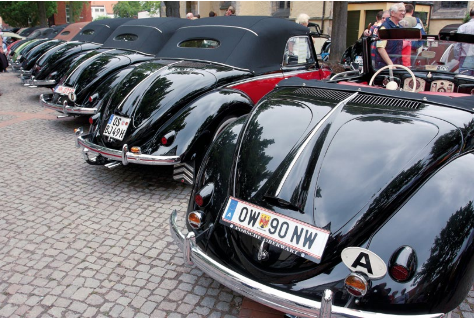
This group of Hebmüller Cabriolets is pictured in the summer of 2009 at a Volkswagen event in Germany. Hebmüllers have distinctive engine compartment covers and centre registration plate lamps. (Courtesy Ken Cservenka)
