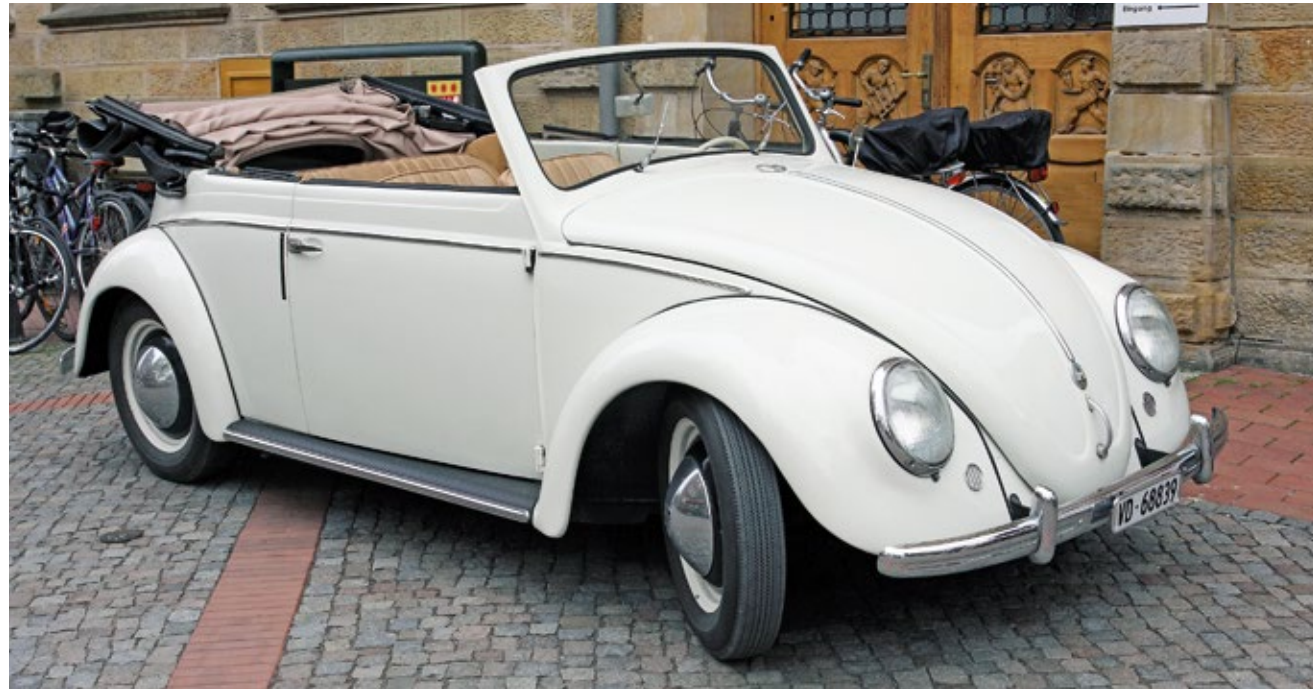
This early Cabriolet depicts models known within VW circles as the 'Split Era.' It dates from before October 1952, as after that date, Cabriolets were given oval instead of round horn grilles, and headlamps were of Volkswagen build instead of the later Bosch type. (Courtesy Ken Cservenka)
