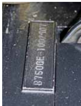
Engine number on top of crankcase behind engine.
