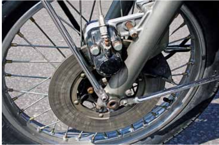
Partially seized brake caliper is a common fault.
